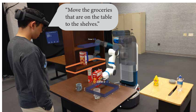
Fig. 1: MARCER, a multimodal robot programming system that combines natural language and augmented reality to build trigger-action rules. A large language model combines commands such as “Move the groceries on the table to the shelves” with environmental context to generate reactive robot programs. AR allows users to set constraints and preview actions through digital twins, directly in their workspace.
