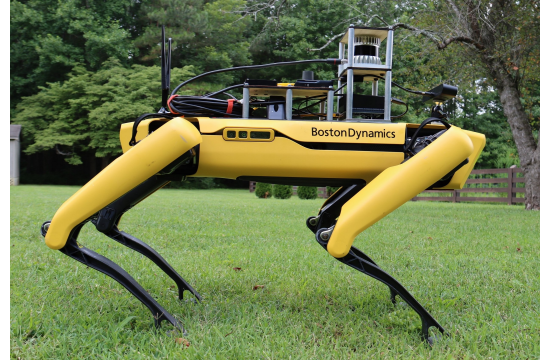
Figure 2: Our quadruped robot with an onboard 360° LiDAR and front-facing stereo camera.
